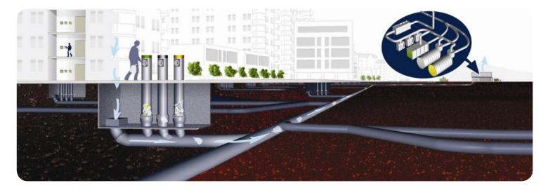
A vacuum waste system is collecting the residual waste in your area. The only thing you can see of the system is the garbage inlets. The picture above shows how a vacuum waste system works.
